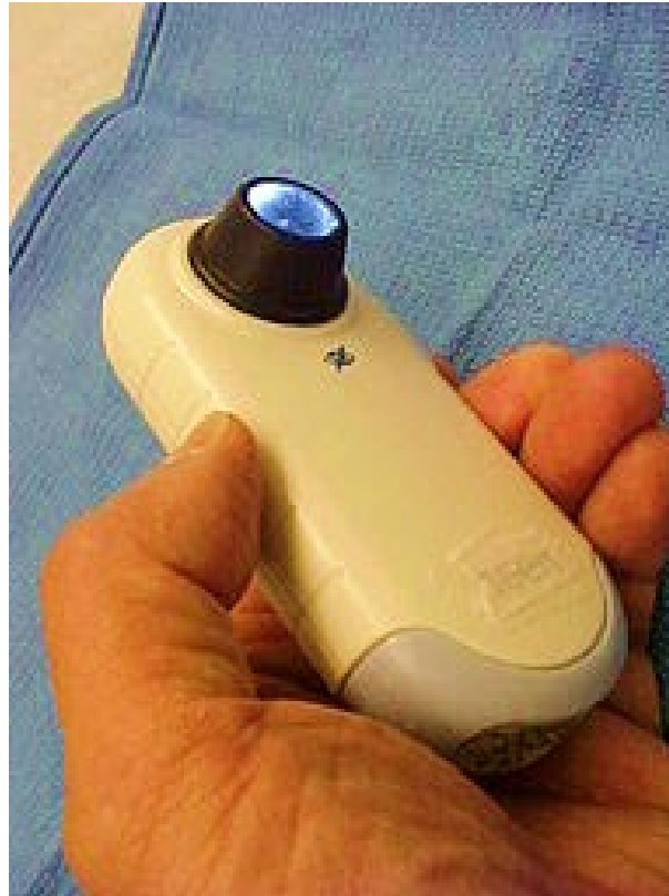
Figure 2 – Modern dermatoscope with double polarized light made by 3GEN.
