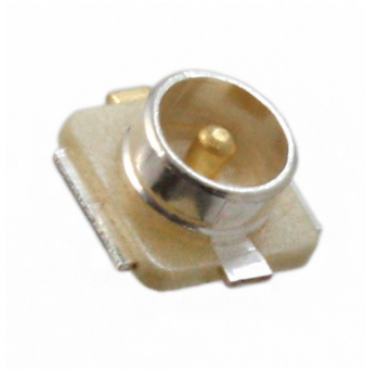
Figura 10 – Conector U.FL Series.
