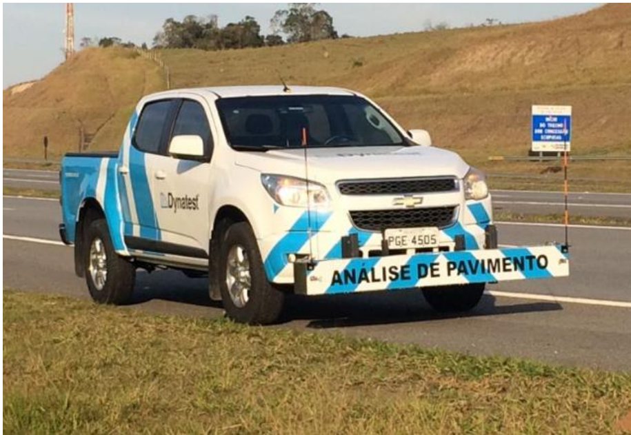
Figura 3.8 – Perfilômetro a laser Dynatest RSP (Dynatest, 2018)
