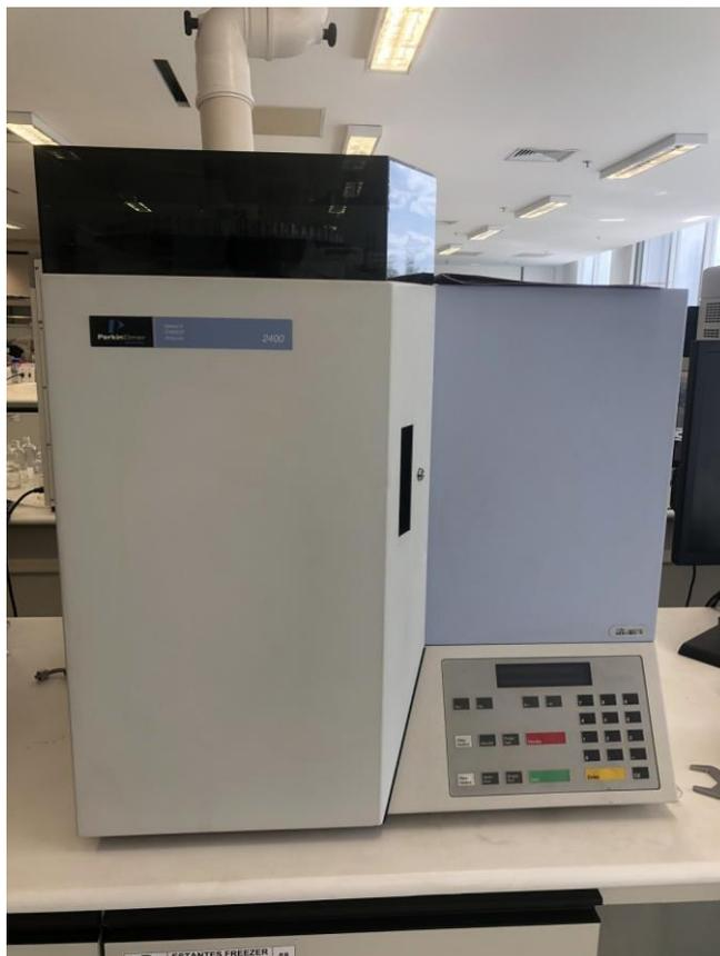
Figura 10. Analisador elementar CHNS/O PE2400 Series II PerkinElmer
