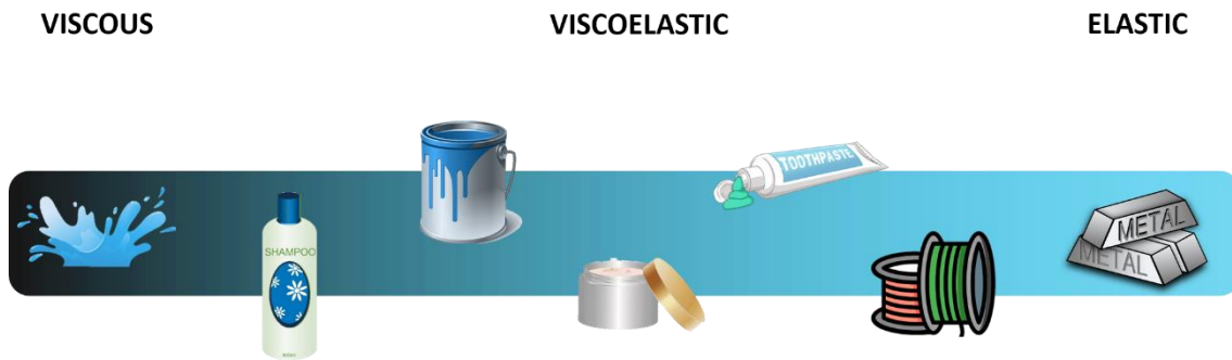
Figure 1.3 Representation of the material's classification according to its deformation response, viscous, elastic or viscoelastic.
