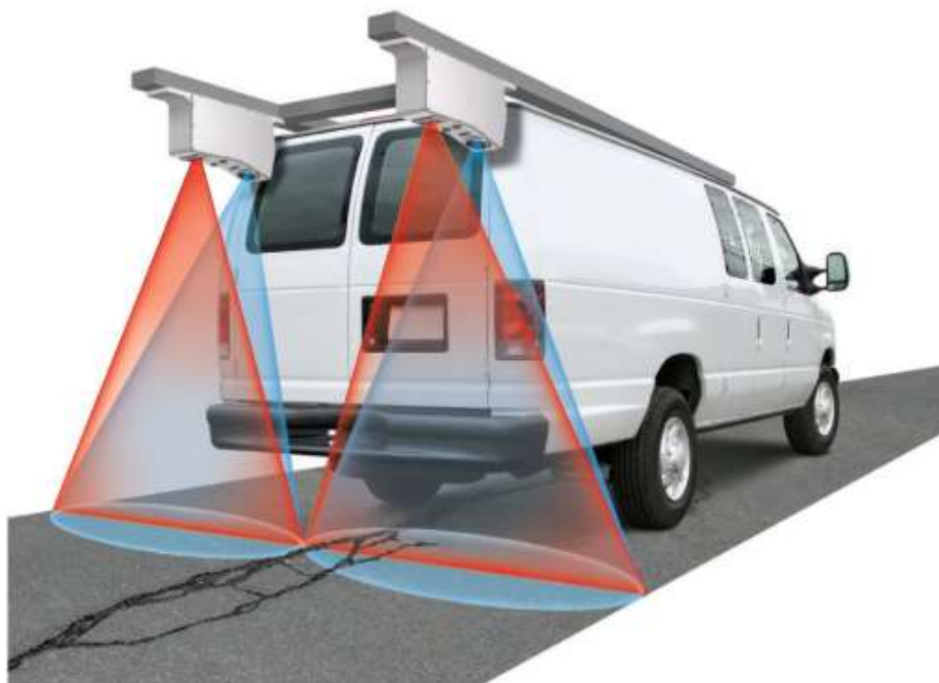
Figura 2.6 - Pavement Scanner (Pavemetrics, 2020).
