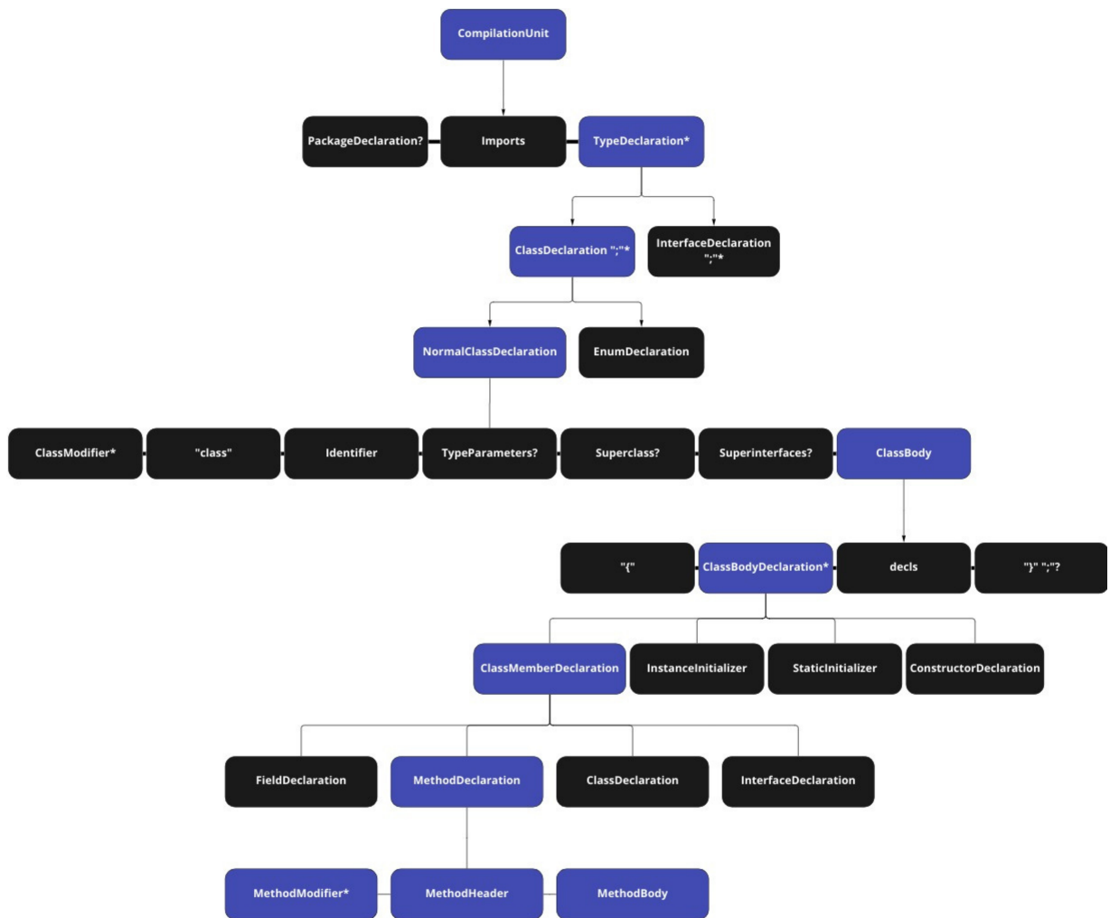
Figure 3.1: Syntax definition tree with highlighted nodes to show the path from CompilationUnit to MethodDeclaration
